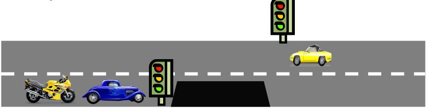
$\lambda_1 = 300$  vehicles per hour  $\mu_1 = 1800$  vehicles per hour  $r_1 = 8$  seconds red time  $\lambda_2 = 600$  vehicles per hour  $\mu_2 = 1800$  vehicles per hour  $r_2 = 8$  seconds red time
