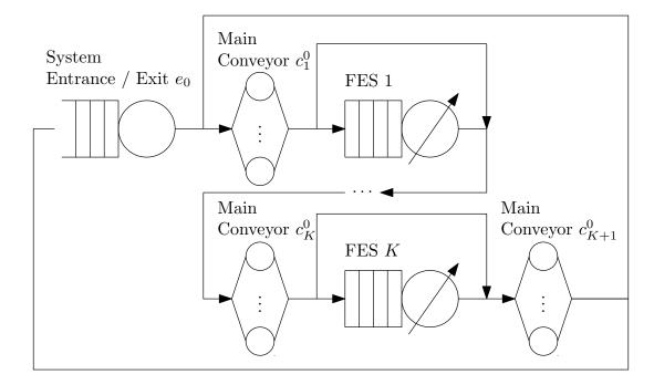
Segments replaced by flow equivalent servers
