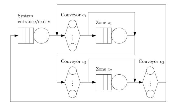
Closed queueing network with  $C = \{c_1, c_2, c_3\}$  and  $Z = \{z_1, z_2\}$
