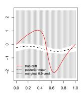
Simulated diffusion data on [0, 100], using the red curve as drift function. Left: hierarchical, right: fixed scale.
